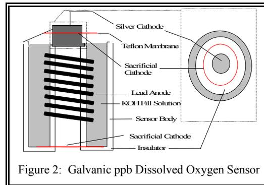
potassium hydroxide (KOH) as the electrolyte. The chemical reactions within the cell are as follows:
