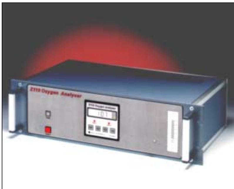
The Z110 zirconia oxygen analyser measures oxygen concentrations from percentage levels to a fractions of parts per million (ppm) in clean gases. Packaged on a 19" rack mounting enclosure, it uses a zirconia oxygen sensor to provide accurate measurement with minimal interference from other gases. The unique cell and heater design gives very fast warm-up times, rapid response, and long sensor life. A wide choice of sampling options is provided to produce virtually 'custom-built' systems.
