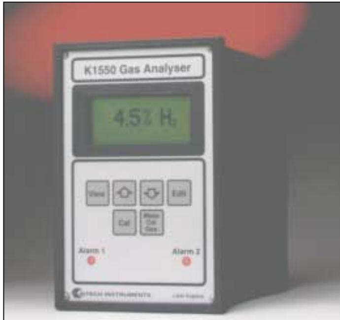
The Hitech K1550 accurately measures the changes of one constituent in binary or pseudo-binary gas mixtures (ie, mixtures in which only one constituent changes). Examples include hydrogen, carbon dioxide, argon, helium and various halogenated hydrocarbons such as the Freons. Almost any single constituent of a gas mixture can be measured providing its thermal conductivity differs from that of the other components. Ranges from high ppm to 100% are possible depending on the gas being measured.
